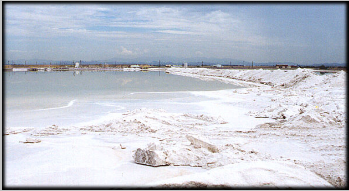
Evaporation pond and piles of salt at the Morton Plant in Glendale, Arizona
